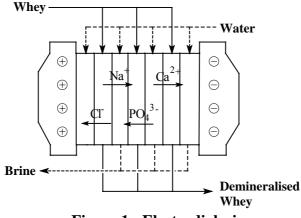
**Figure 1 - Electrodialysis**
